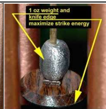
Close up for tapered edge wood striker with weight & axle
